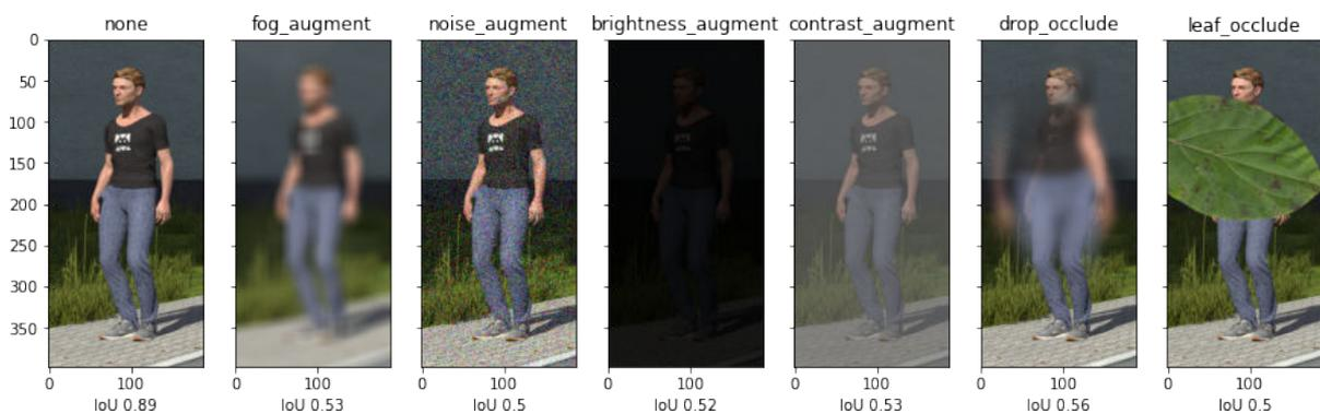
Figure 6: Examples of augmented images, using different augmentation algorithms. Left-most: The original image. All augmenters were calibrated to inhibit the AI to a similar degree.
